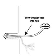
more dust blows out. This stage is easier if you have a source of compressed air or a vacuum cleaner to suck the dust up (a crevice tool and the plastic tube can work well), but take care to protect your eyes and avoid breathing the dust, however you clean the holes.
